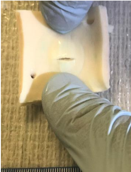
Experiment 8: 4.53 mm with circumferential rupture (lumen, adventitia)
