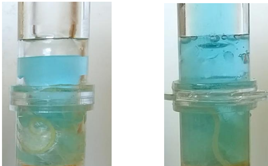
Figure 29 (a) Compliant balloon filling the upper chamber (b) compliant balloon with a silicone sample filling the upper chamber.
