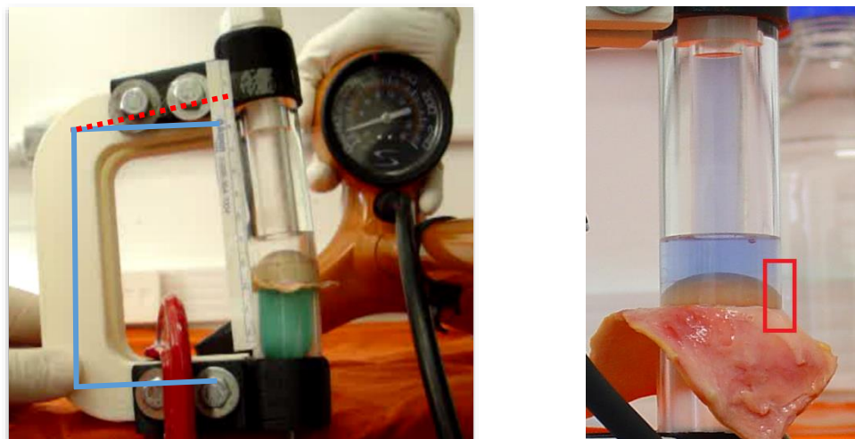
Figure 22: BIT clamp module failure, slipping and pressure attenuation.
