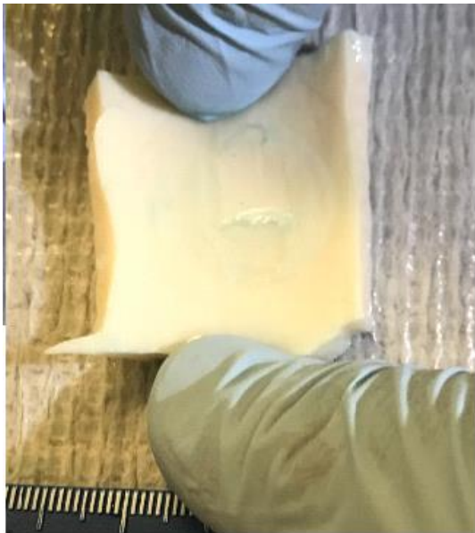
Experiment 6: 3.94 mm with circumferential rupture (lumen, adventitia)
