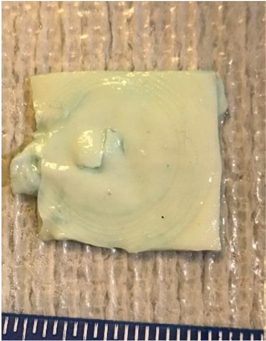
Experiment 4: 2.26 mm with circumferential rupture (lumen, adventitia)
